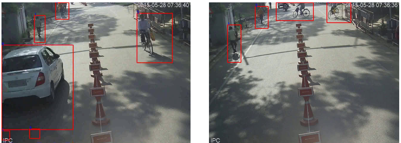
Figure 4: Objects detected and tracked in the video after applying background subtraction(mog2), and subsequent calculation of bounding boxes.
