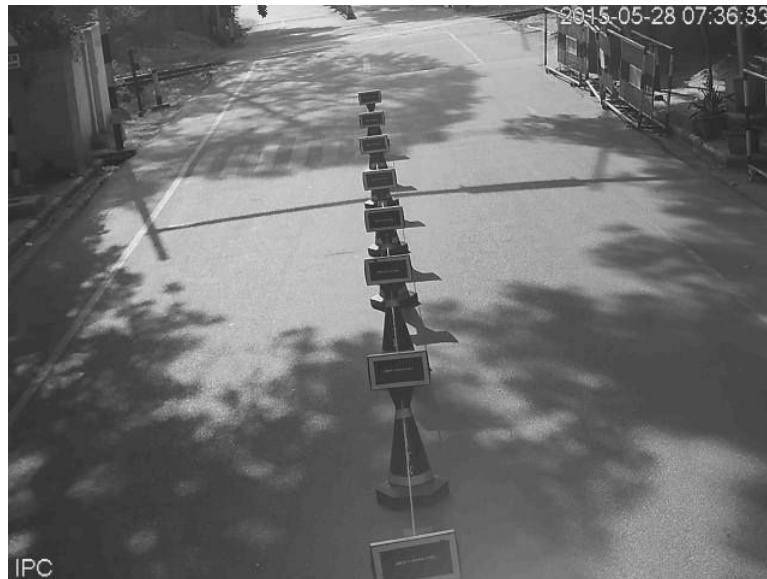
Figure 2: Background image calculated using the mode of pixel intensity.
