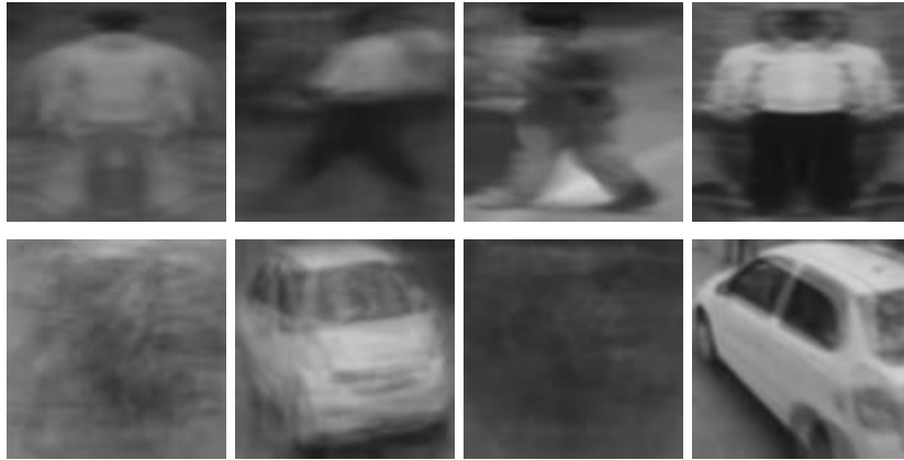
Figure 5: Class representatives of person and vehicles obtained by doing K-means clustering.
