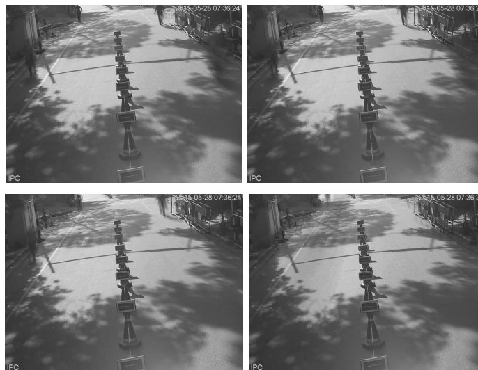
Figure 1: Clockwise, the background images calculated by averaging 10, 20, 40 and 200 frames.
